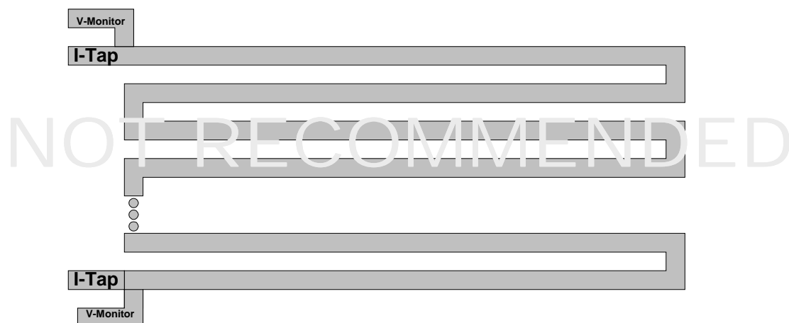
Figure 6 — Example Kelvin connected, serpentine SIV structure, without bridging monitor lines . This variation is Not Recommended .
